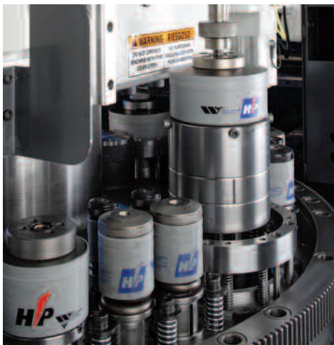
A fixed 114,30 mm station accommodates large parting tools, louvers or special forms.
