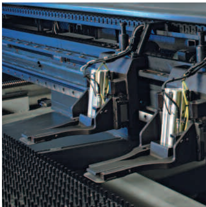
Programmable work clamps reduce or eliminate no punch zones.
