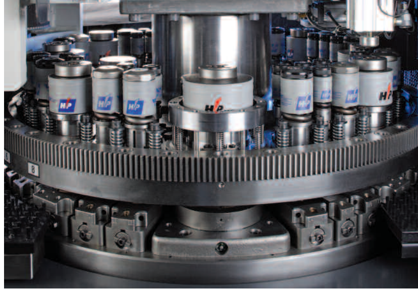
The large capacity turret features up to 48 stations.
