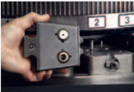
Quick-change die holders reduce set-up time to increase overall productivity.
