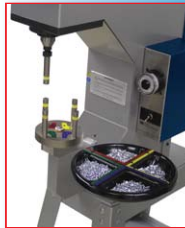
Round turret installed on an LT/4 press.
